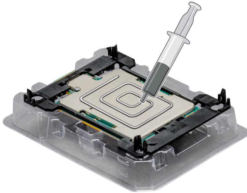
Figure 35. Applying thermal grease on top of the processor
